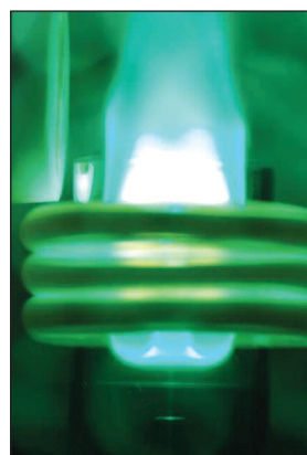
Figure 2: The plasma aspirating naphtha after the auxiliary and nebulizer gas flows have been optimized.
