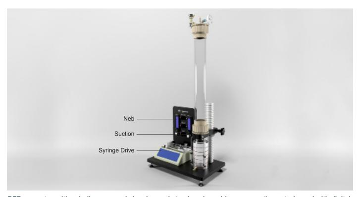
BFE apparatus with nebulizer, aerosol chamber and stand, syringe drive, pneumatic control panel with digital flow meters, cascade impactor, vacuum pump and petri dishes.
