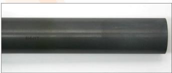
By contrast, the ceramic material does not devitrify and is not affected by salt deposits. The ceramic D-Torch in the photo was run for the same period and with the same samples as the quartz torch but shows no degradation at all.
